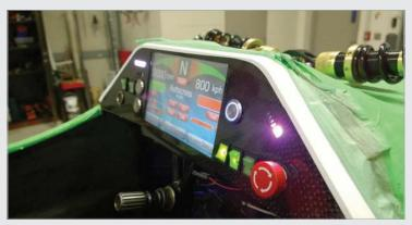
**Above** The Raspberry Pi 2 sits behind the dashboard and powers the display. When the car is racing, it automatically sends telemetric data to the team in the pits
