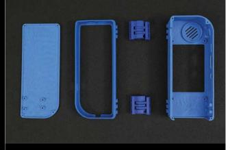
Above The 3D-printed case, complete with modular hinges
