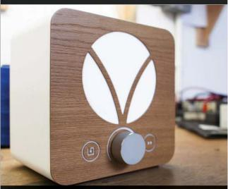
Above Capacitive touch sensors are used for the 'skip' and 'save' buttons
