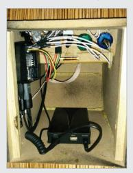
**Above** A hollowed-out interior houses the Raspberry Pi and the wires for the authentic arcade parts
