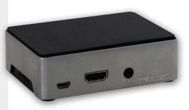
The Flirc Case has a very solid construction as it's made from a solid aluminium shell with a matte, rubberised plastic top and base. The aluminium finish gives the case a premium feel, too, which is always a bonus. Unlike the other cases on test, it comes with a built-in heatsink. It's easy to put together, using four screws to secure it.
