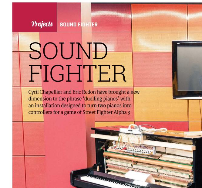
e seamlessly transformed two classical upright pianos into PlayStation 2 controllers using custom analogue piezo triggers, a Pi B+, and Arduino Unos, and created a specific Python 3 firmware to map a classical playing style onto the Street Fighter Alpha 3 gameplay, including combos and the like," explain the French duo.
